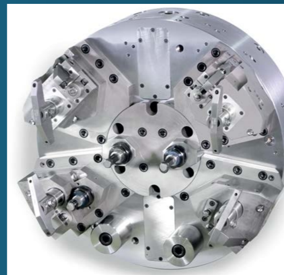
Realisation of two subsequent operations in one chuck
